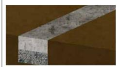
Fill concrete, 3 parts sand + 1 part water + 1 part cement, into the base of the trench.
